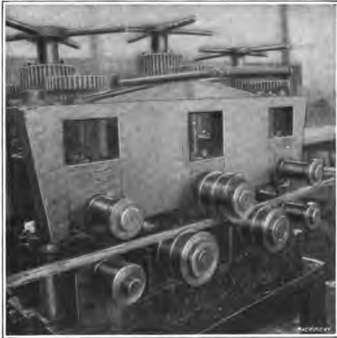
Fig. 13. Machine for Straightening Square, Hexagonal, Octagonal, and Flat Bars
